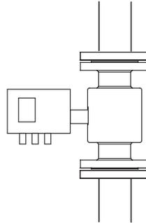
Figure 6: Vertical placement
