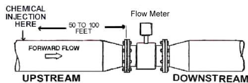
Figure 11: Chemical injection point upstream of meter
