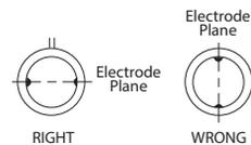
Figure 7: Horizontal placement
