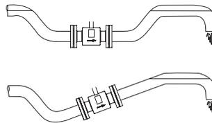
Figure 14: Pipe positioned to keep water in detector
