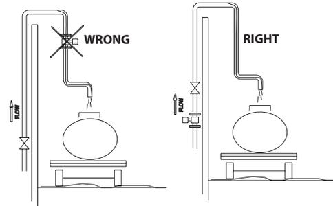
Do not install in a vertical, downward position.
