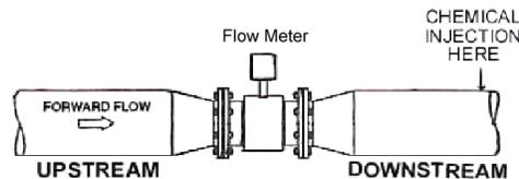
Figure 10: Chemical injection point downstream of meter
