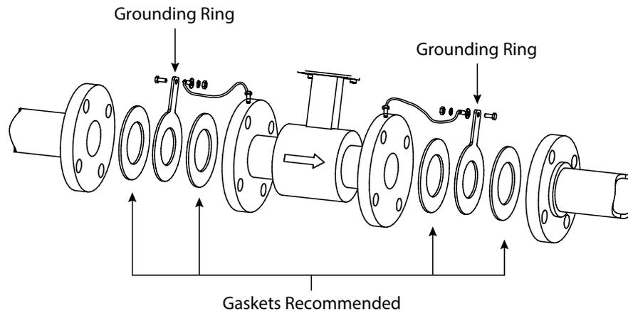
Figure 15: Meter/pipeline connection gaskets and grounding rings
