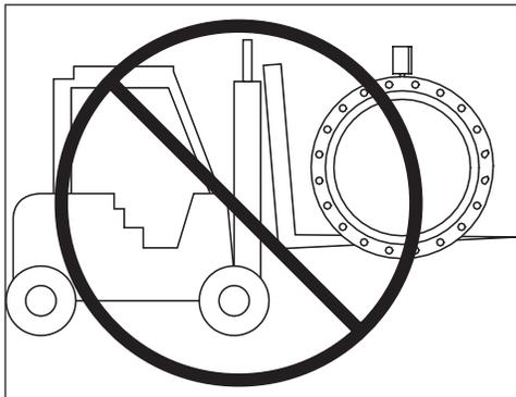
Do not lift detector with forklift.
